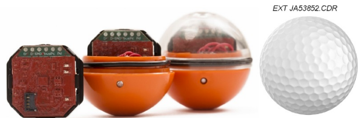
Figure 9. Pipers sensor (courtesy of Ingu Solutions).
